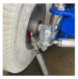
4. To adjust the chain tension, use a flat head screw driver to push down slightly on the sprocket shaft and a 15/16 wrench to loosen the nut. Chain should be fairly taut with minimal play.
